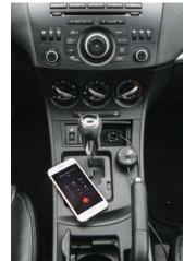
dashboard, or any surface facing the driver then connect the 3.5mm audio connector to the auxiliary input port and power it through the included USB/CLA power adapter, (the CLA also includes a secondary USB receptacle with 2.1 amp smartphone charging support). For cars not equipped with an auxiliary input, the BCS1 can utilize any of the Audiovox OEI Silverline DUO vehicle specific interface modules or the AUNI150PRO universal interface module (sold separately).
