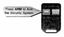
To arm the system, exit the vehicle, close all doors, then press and release the ARM button.
