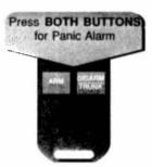
Pressing both buttons together on the remote transmitter activates the Panic feature, sounding the siren and flashing the parking lights. Panic is designed to bring attention to the vehicle and surrounding area, warding off a would-be intruder. Press either button on the remote transmitter to turn off the Panic alarm.
