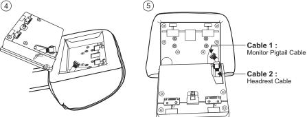
Match M1 monitor pigtail cable to M1 headrest cable Match M2 monitor pigtail cable to M2 headrest cable
