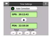
Turn on the Auto Correction switch to let The NVX200 Navigator frequently check and correct the PND time with the GPS time.
