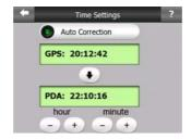
Turn on the Auto Correction switch to let Touch & Go Navigator frequently check and correct the PND time with the GPS time.
