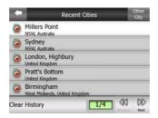
Should the settlement you are looking for appear on the list, just tap it and you will immediately jump to the Street Name Input screen with the selected city name or postcode shown at the top of the screen. If the desired settlement is not displayed, use the arrows in the bottom right corner to see more of this list.
