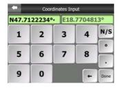
When you enter this page, the coordinates of the current GPS position (or the selected map point (Cursor) if Lock-to-Position is inactive) are shown at the top of the display.
