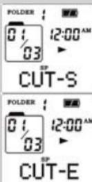
Tips: Cutting, inserting new segments and adding appendix will only update the recorded time length, without changing recording time and date.
