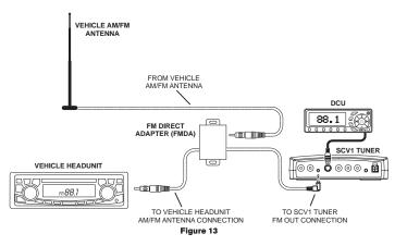
To hear the SIRIUS audio, the vehicle's headunit and the SCV1 will need to be tuned to the same FM channel. Refer to the *FM Transmitter* section on page 56 for more detailed instructions on how to tune the SCV1 to an FM channel.
