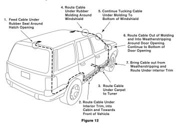
Installing the FM Direct Adapter
