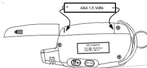
4. Replace battery cover by sliding into it's original location until it is fully seated.
