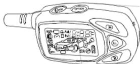
**NOTE:** Transmitter must be within operating range of the vehicle, approximately 1000 ft.
